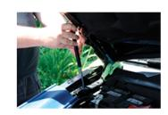
STEP 4-Place masking tape alongside upper hood hinges and mark location of bolts to ensure proper hood realignment
