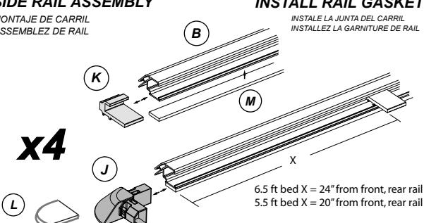
Assemble rails by inserting Bow Slider into side rails, followed by an Endcap.
