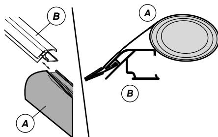
Slide into extrusion from end.
