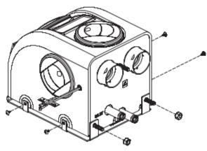
SECURE BRACKET TO HOUSING WITH FOUR #8 SCREWS PREVIOUSLY REMOVED AND TWO 5/16-18 NUTS.
